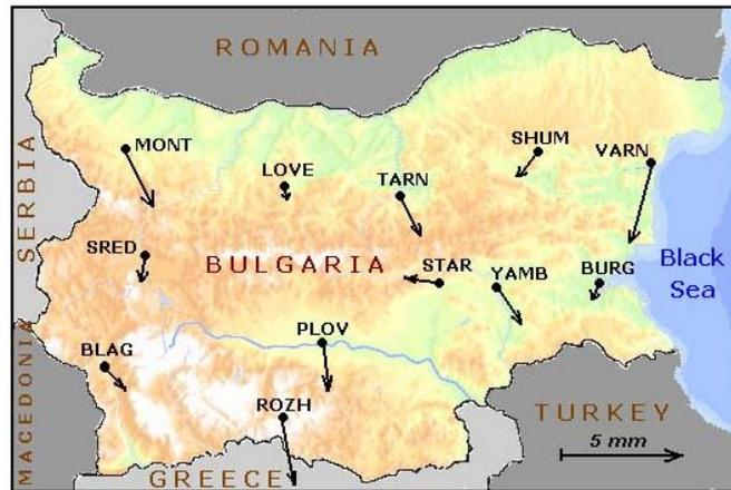
Fig. 6: ETRF2000 horizontal velocities of BULiPOS network stations
