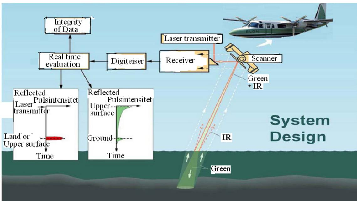
Fig.10. System for simultaneous scanning of underwater topography and land BLOM]
