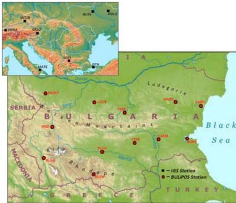
Fig.5: Location of BULiPOS network stations (in red) and IGS reference stations introduced (in black)
