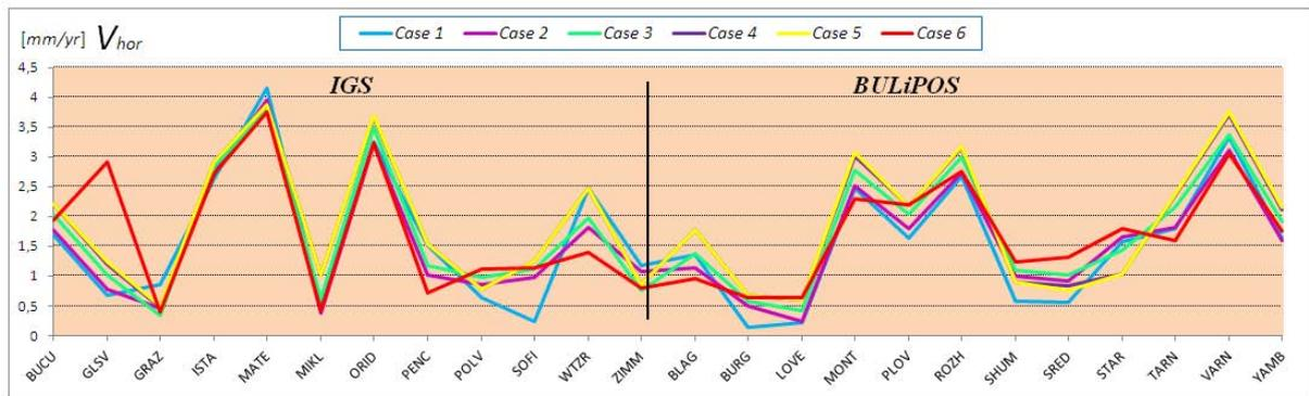
Fig. 7: Comparison of the horizontal velocities of the IGS and BULiPOS stations in ETRF2000
