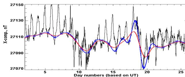
*Fig.4. X-component series for 25 days of the HON station, centered on 03 February 2008. The midnight points (24 LT) are marked by blue "x" sign. The computed spline through the midnight points is drawn by a continuous blue line, the smoothed spline by a red line. The result is very close to the one of McPherron. (Compare Fig. 5a in McPherron and Chu.)*
