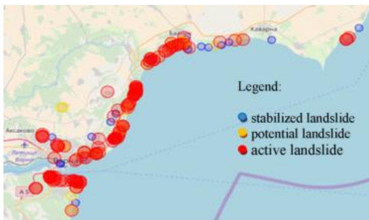
Fig. 1. Map of active, stabilised and potential landslides in NE Bulgaria (according to GIS of the Ministry of Regional Development and Public Works (MRDPW) ( http://gis.mrrb.government.bg/ ))
