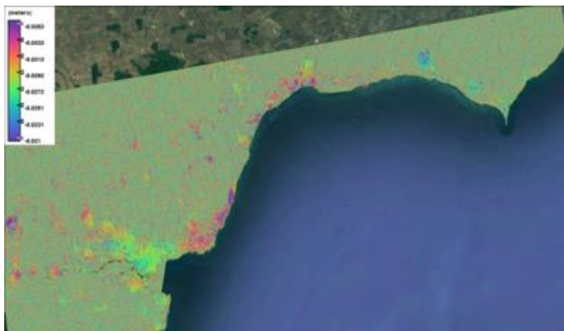
Fig. 4. Ground displacements obtained from the IFI Jan 1st 2015 – Dec 21st 2016
