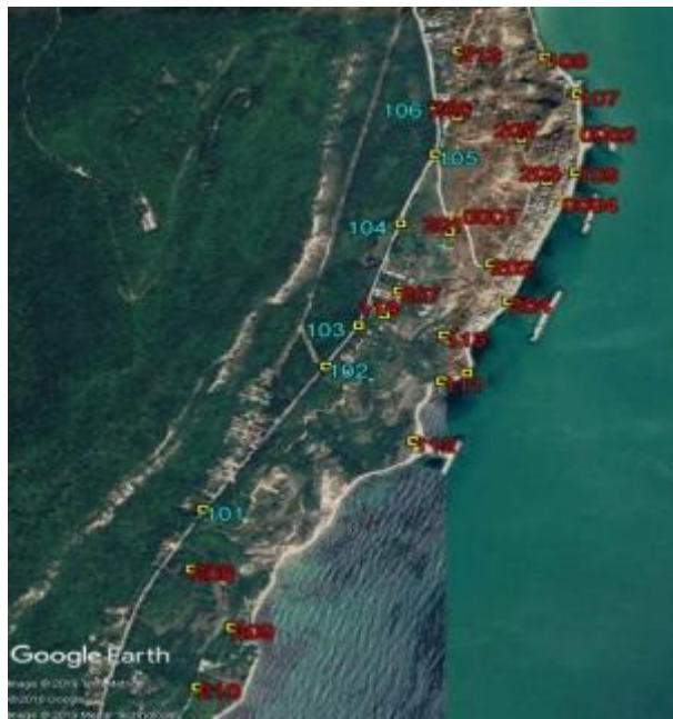
Fig. 8. Points of the new geodynamic network in and around the landslide "Dalgiya yar"
