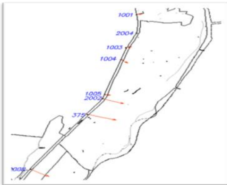
Fig. 9. Horizontal displacements for the period 2018–2013
