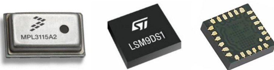
Fig. 4. ICs engaged in Z-Pilot Nano as sensors. From left to right: Digital barometer MPL3115A2; Digital IMU – LSM9DS1 top view; LSM9DS1 bottom view.
