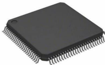
Fig. 3. NXP Digital Signal Controller implemented as the main IC in Z-Pilot Nano. The used variant is installed into an SMD LQFP 100-pin package with dimensions 14×14 mm.
